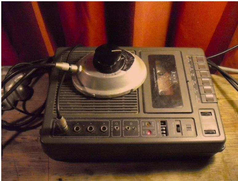
Figure 4: “Pie-dish oscillator” and amplifier made from discarded objects (Felix Modregal)
